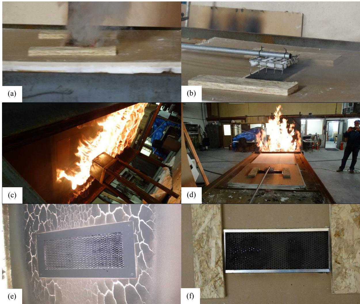
Figure 12. Test 5 showing (a) smoke through vent, (b) cotton 1, (c) flames under table, (d) flames out back end, (e) vent front, and (f) vent back.
