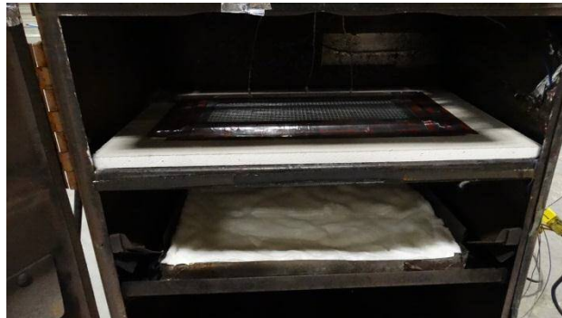
Figure 2. Actual installation of vent in ember chamber with upper and lower shelf.
