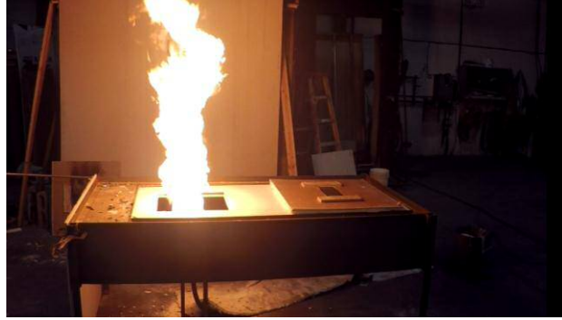
Figure 4. Actual flame prior to horizontal vent test.
